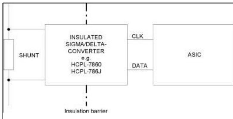
Figure 2: Block diagram/principle sketch of the current measurement using a shunt.
