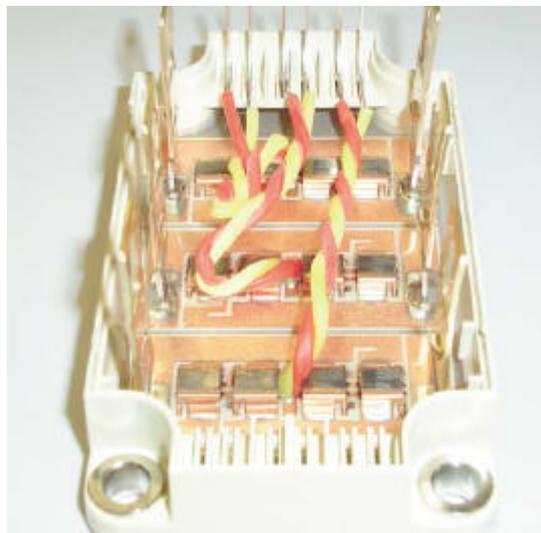
Figure 1: Shunt module for use in large converters of Siemens AG. It was developed in cooperation with Isabellenhütte (shunts) and Semikron (module housing).
