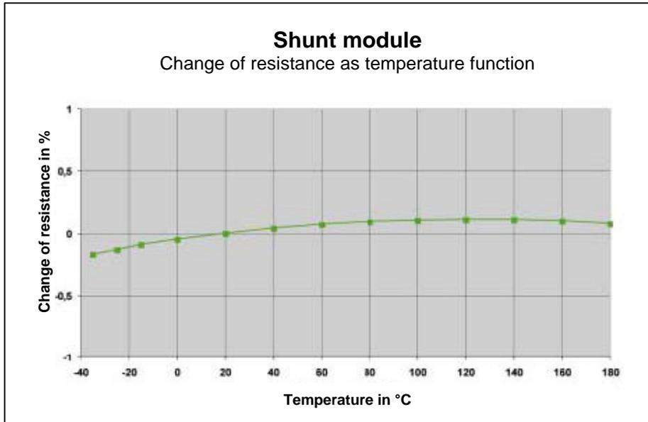
Figure 4: Change of resistance of shunt module as temperature function
