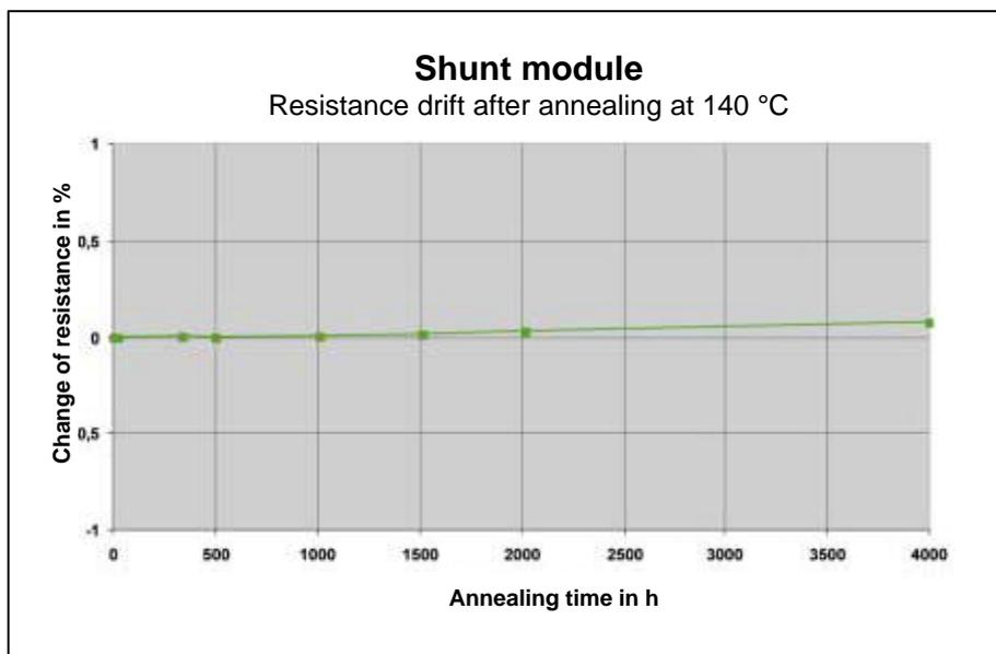
Figure 5: Resistance drift of shunt module after annealing at 140 °C.
